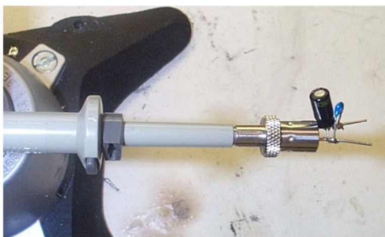
Figure 42 – Oscilloscope Probe with Probe Master ( www.probemaster.com ) 4987A BNC Adapter. (Modified with wires for ripple measurement, and two parallel decoupling capacitors added)
