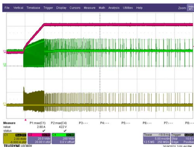
Figure 37 – Flyback Start-up Waveforms, 160 VAC Input, 0 A Load. Red – V_{OUT} , 20 V / div. Grn – U1 V_{DRAIN} , 200 V / div. Yel – U1 I_{DRAIN} , 2 A, 5 ms / div.
