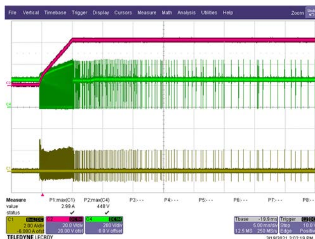
Figure 38 – Flyback Start-up Waveforms, 180 VAC Input, 0 A Load. Red – V_{OUT} , 20 V / div. Grn – U1 V_{DRAIN} , 200 V / div. Yel – U1 I_{DRAIN} , 2 A, 5 ms / div.
