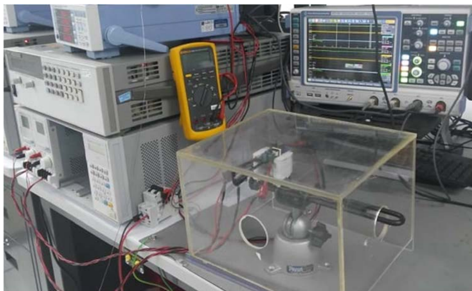
Figure 136 – Thermal Performance Set-up Using an Acrylic Box.
