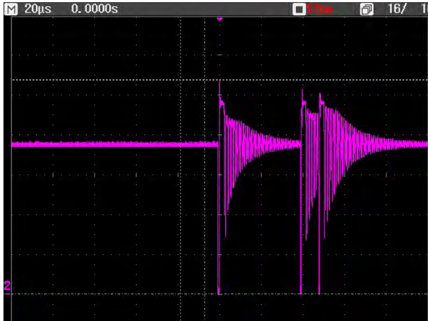
Vin=264 Vac, Vout=20 V, Iout=0A Vds_pri (max) = 535V
