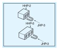
Figure 6. Terminal Jumper Description
