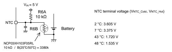
Figure 14. Resistor Setting of NTC Terminal
