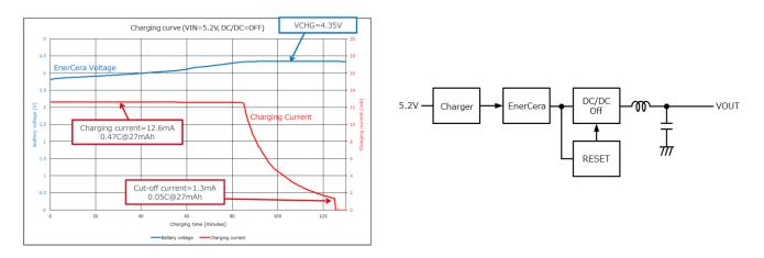
The charging time should be used as a guide. (It is not charging from a full discharged state.)
