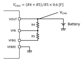
Figure 10. Resistor Setting of VCHG
