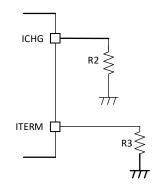
Figure 12. Resistor Setting of ICHG and ITERM
