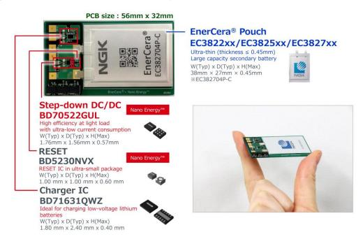
Figure 2. Products Mounted on Collaboration Board
