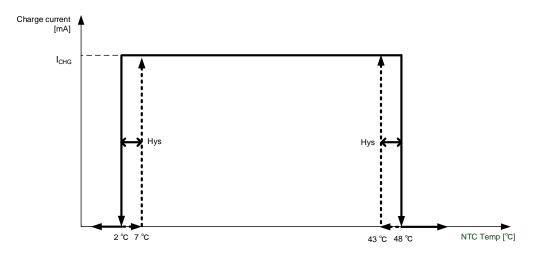
Figure 13. Charge Current vs Battery Temperature
