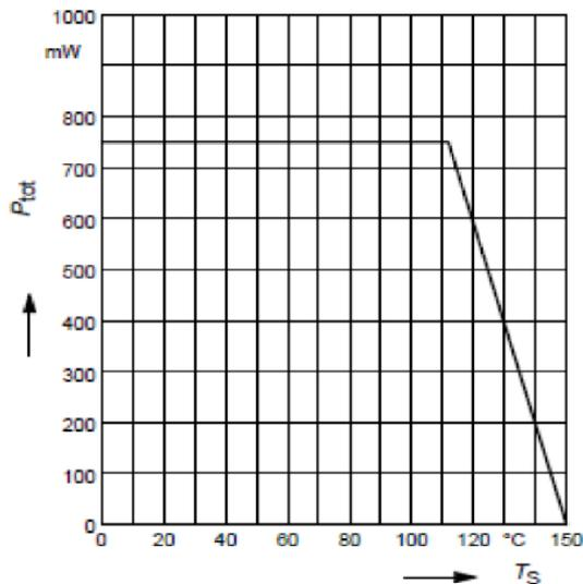
Fig.1 Permissible total power dissipation  $P_{tot} = f(T_s)$
