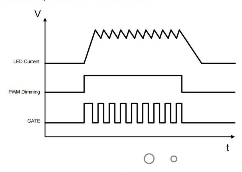
The rising and falling edges are limited by the current slew rate in the inductor. The first switching cycle is terminated upon reaching the 250mV (V<sub>DIM</sub> • 0.167) level at CS. The circuit is further reaching its steady-state within 1 switching cycles regardless of the switching frequency.
