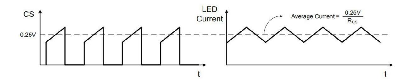
The above equations are only valid for continuous conduction of the output inductor. It is a good practice to design the inductor such that the switching ripple current in it is 25% of its average peak-to-peak, full load, DC current.
