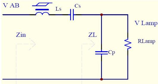
$$\text{電路增益為 } \frac{V_{\text{Lamp}}}{V_{\text{AB}}} = \frac{Z_L}{Z_{\text{in}}}$$
