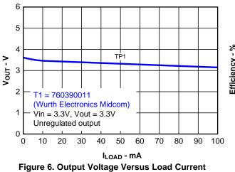
90 80 70 Efficiency - % 60 50 40 30 T1 = 760390011(Wurth Electronics Midcom) 20 Vin = 3.3V, Vout = 3.3V 10 Unregulated output 0 10 20 30 40 50 60 70 80 90 100 I<sub>LOAD</sub> - mA
