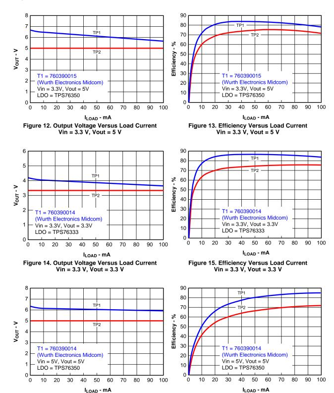
Figure 16. Output Voltage Versus Load Current
