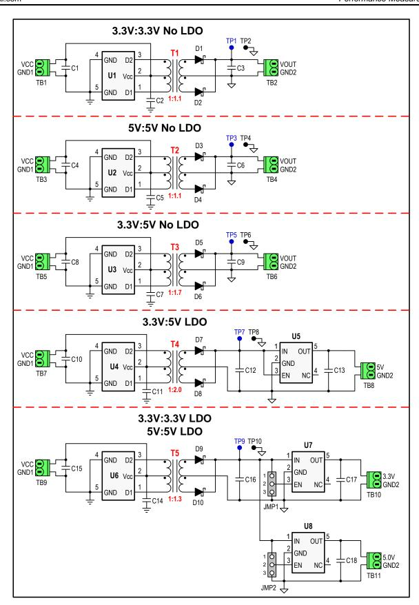
Figure 3. SN6501 EVM Schematic
