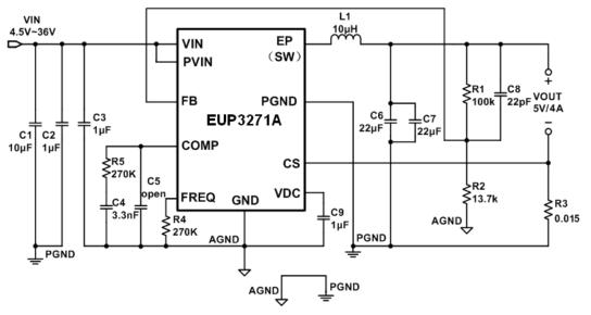
Figure 2. 340KHz Operating Frequency Application Circuit
