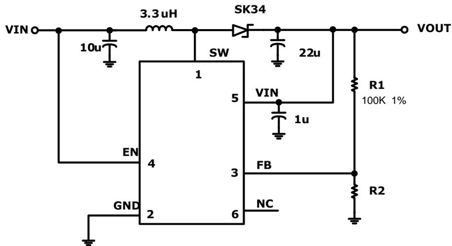
$$V_{OUT} = V_{FB} \times \left(1 + \frac{R1}{R2}\right)$$
