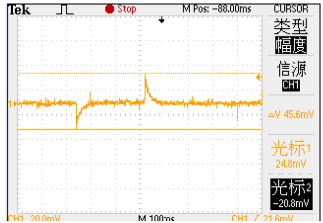
6. 纹波抑制(IL=50mA, Vpp=1V, F=10KHZ)
