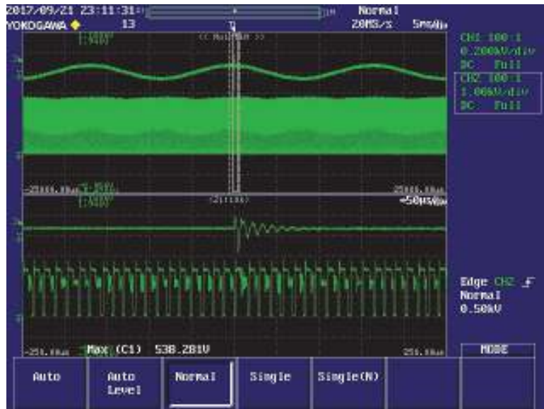
Figure 97 – (+) 2.5 kV Ring Wave Surge. 90° Phase Angle, Input: 230 VAC. V_{DRAIN} , 200 V / div., 20 ms / div. Peak V_{DRAIN} : 558.333 V.
