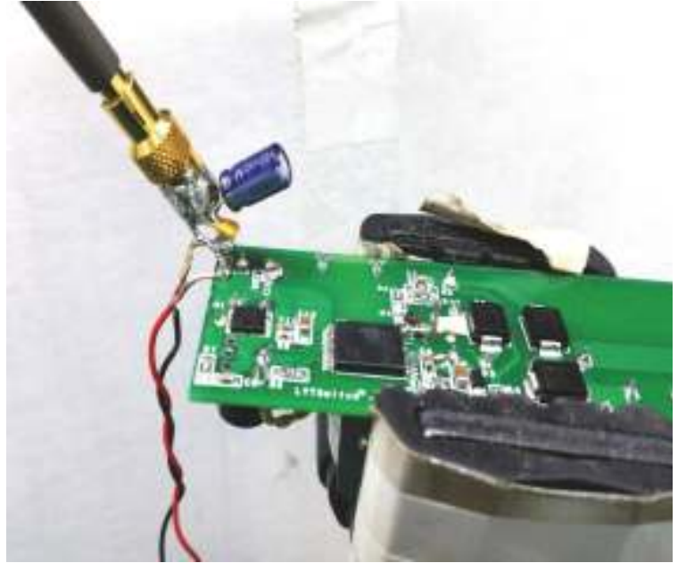
Figure 77 – Unit Set-up for Output Voltage Ripple Test.
