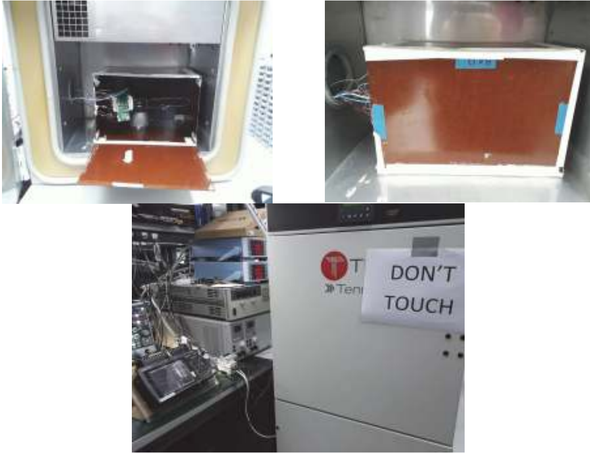
Figure 23 – Test Set-up Picture Thermal at 60 °C Ambient - Open Frame.
