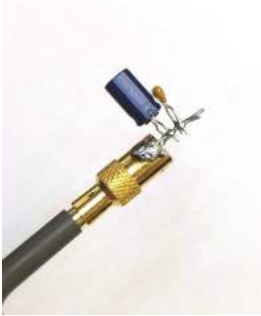
Figure 76 – Probe Set-up for Output Voltage Ripple Test.
