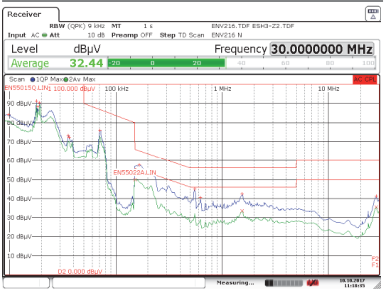
Figure 93 – Conducted EMI QP Scan at Full Load, 230 VAC 60 Hz and EN55015 B Limits.
