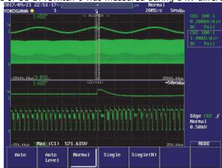
Figure 95 – (+)1 kV Differential Surge. 90° Phase Angle, Input: 230 VAC. V_{DRAIN} , 200 V / div., 20 ms / div. Peak V_{DRAIN} : 571.615 V.
