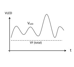
By cascade mode, two or more NU502 in series can absorb higher voltage variation in lighting system. Each NU502 can share about 12 volts redundant. The total voltage variation range that system can work is calculated by following equation.
