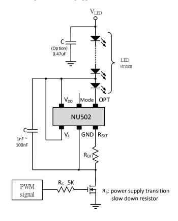
• DC PWM dimming application (No leakage current)
