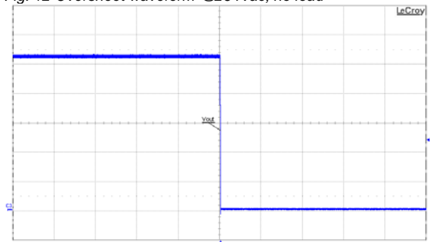
Fig. 12 Overshoot waveform @264Vac; no load
