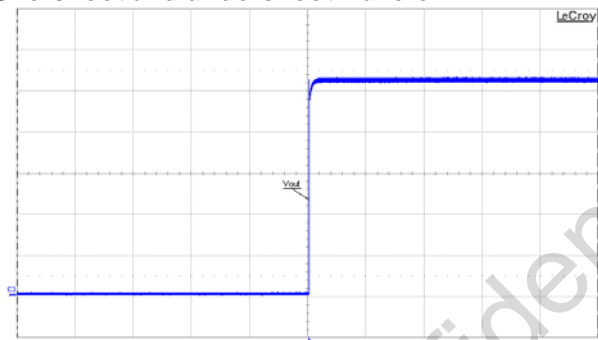
Fig. 9 Overshoot waveform @90Vac; full load
