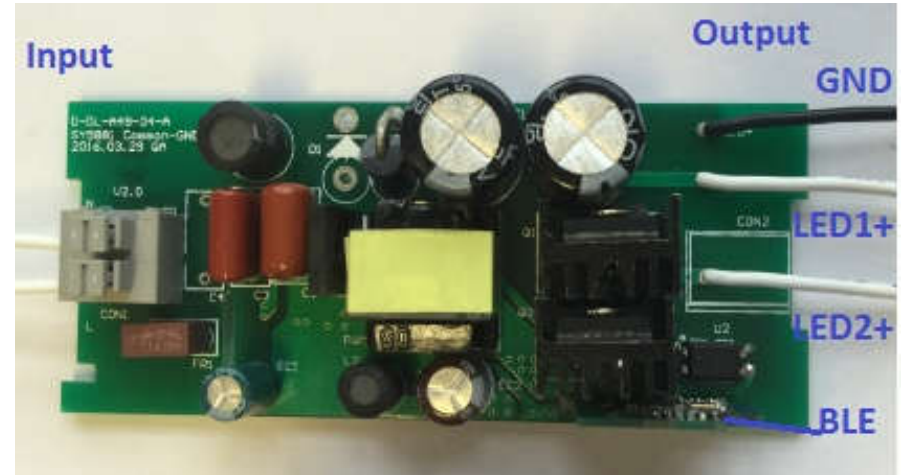
SY5881 25W Warm/Cold dimmable Fixture EVB
