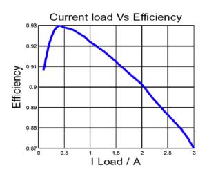
Figure 2: Efficiency Curve for Vout=5V
