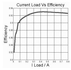
Fig 3 Efficiency Vs Light Load
