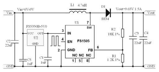
For Vin=6V~9V Vout=9.65V 1.5A efficiency≥90%
