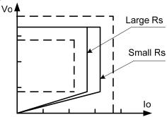
Figure.3. Adjustable output power by changing Rs
