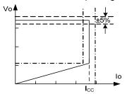
Figure.1. Typical CC/CV Curve
