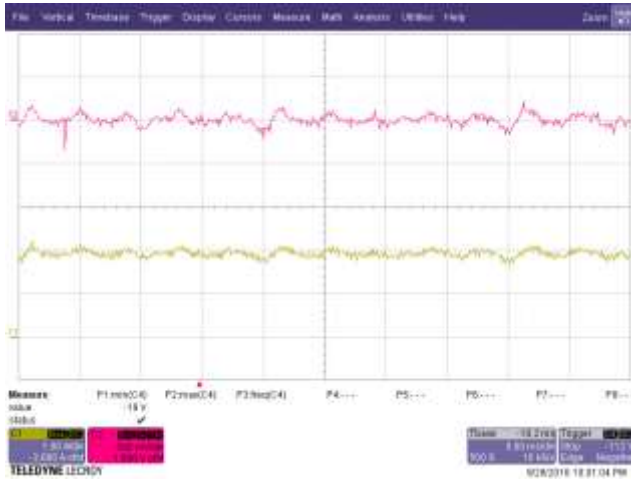
Figure 28 – Main Output Voltage and Current Ripple in CC Mode, 180 VAC, Chroma CV Load, 30 V Setting. Upper: Main V_{OUT(RIPPLE)} , 500 mV / div. Lower: I_{OUT(RIPPLE)} , 1 A, 5 ms /div.
