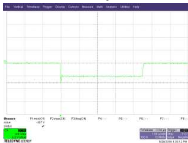
Figure 17 – Output Rectifier (D3) Reverse Voltage, 230 VAC Input, 100% Load. 200 V, 1 \mu s / div.
