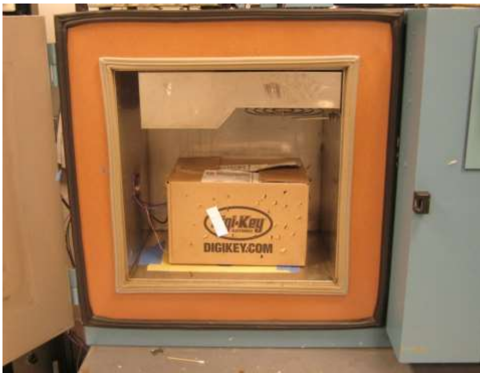
Figure 34 – Isolation Box in Thermal Chamber.
