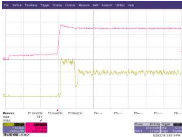
Figure 19 – Output Start-up, CC Mode, 230 VAC, Chroma CV Load, 50 V Setting. Upper: Main V_{OUT} , 20 V / div. Lower: Main I_{OUT} , 1 A, 20 ms / div.
