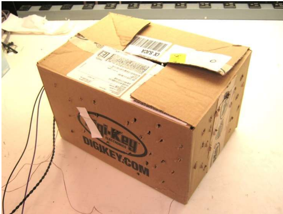
Figure 33 – Isolation Box with Equilibration Holes for Thermal Chamber Testing.
