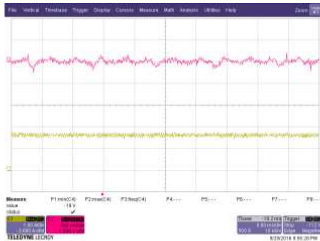
Figure 25 – Output Voltage and Current Ripple in CV Mode, 230 VAC, Chroma CC Load, 1.5 A Setting. Upper: V_{OUT(RIPPLE)} , 500 mV / div. Lower: I_{OUT(RIPPLE)} , 1 A, 5 ms / div.
