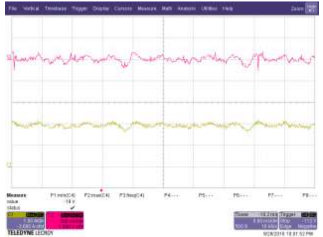
Figure 29 – Main Output Voltage and Current Ripple in CC Mode, 230 VAC, Chroma CV Load, 30 V Setting. Upper: Main V_{OUT(RIPPLE)} , 500 mV / div. Lower: I_{OUT(RIPPLE)} , 1 A, 5 ms /div.
