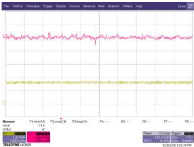
Figure 24 – Main Output Voltage Ripple, 180 VAC, CV Mode, Using Chroma CC Load, 1.5 A Setting. Upper: V_{OUT(RIPPLE)} , 500 mV / div. Lower: I_{OUT(RIPPLE)} , 1 A, 5 ms / div.
