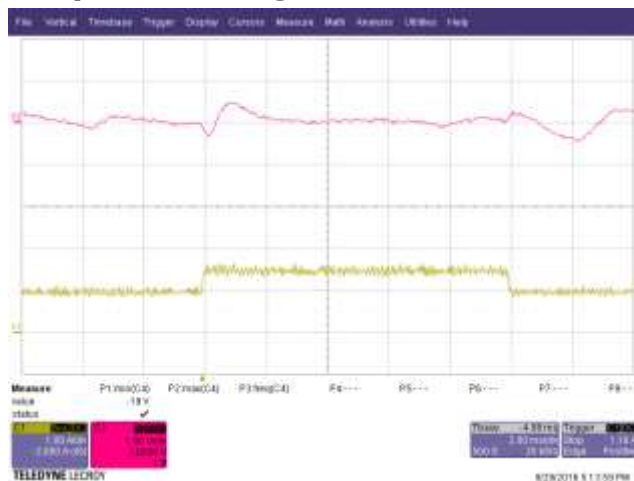
Figure 21 – Output Transient Response, CV Mode, 50%-75%-50% Load Step, 230 VAC Input. Upper: V_{OUT} , 1 V / div. Lower: I_{OUT} , 1 A, 2 ms / div.
