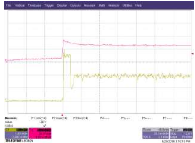
Figure 20 – Output Start-up, CC Mode. 230 VAC, Chroma CV Load, 30 V Setting. Upper: Main V_{OUT} , 20 V / div. Lower: Main V_{OUT} 1 A, 20 ms / div.
