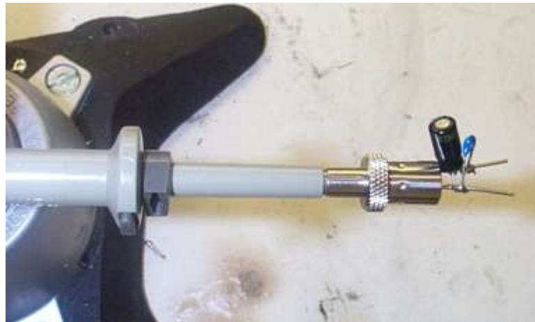
Figure 23 – Oscilloscope Probe with Probe Master 4987BA BNC Adapter (Modified with Wires for Probe Ground for Ripple measurement and Two Parallel Decoupling Capacitors Added).
