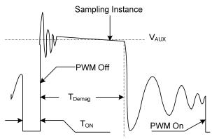
Figure.2. Auxiliary voltage waveform
