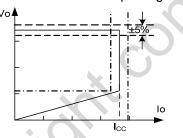
Figure.1. Typical CC/CV Curve
