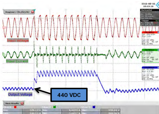
Figure 66 – Line Swell 300 VAC, 100% Load. Upper: V_{IN} , 400 V / div. Middle: I_{IN} , 4 A / div. Lower: V_{OUT} (DC Offset), 50 V / div., 50 ms / div.
