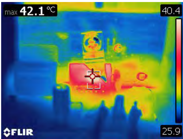
Figure 19 – Infra-Red Images of HiperPFS-4 MOSFET at Thermal Equilibrium, 230 VAC, Full Load, with Forced-Air Flow.
