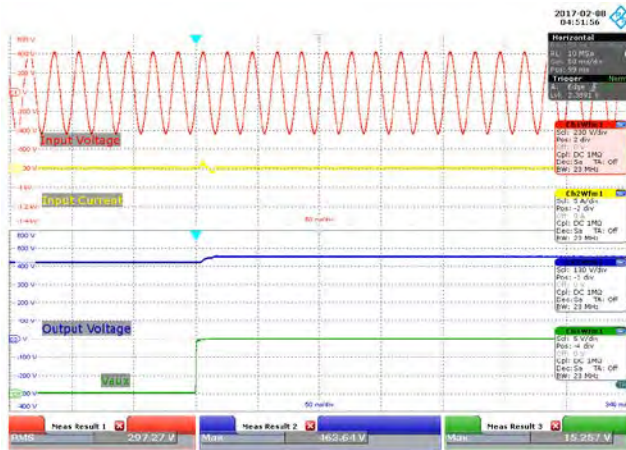
Figure 37 – 300 VAC, No-Load. Upper: V_{IN} , 200 V / div. Second: I_{IN} , 5 A / div. Third: V_{OUT} , 100 V / div. Lower: V_{AUX} , 5 V / div, 50 ms / div.
