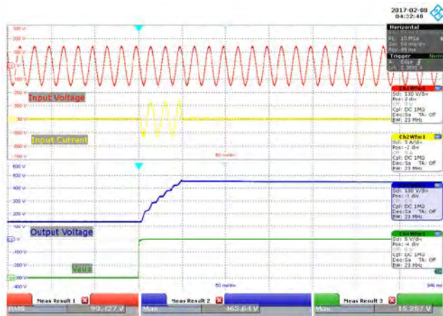
Figure 27 – 100 VAC, No-Load. Upper: V_{IN} , 100 V / div. Second: I_{IN} , 5 A / div. Third: V_{OUT} , 100 V / div. Lower: V_{AUX} , 5 V / div, 50 ms / div.
