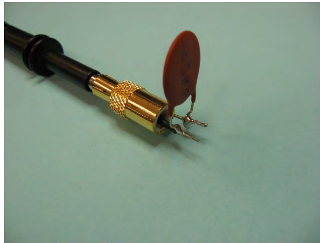
Figure 77 – Oscilloscope Probe with Probe Master ( www.probemaster.com ) 4987A BNC Adapter (Modified with wires for ripple measurement, and one parallel decoupling capacitor added.)
