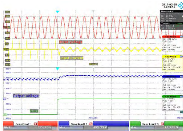
Figure 36 – 277 VAC, Full Load. Upper: V_{IN} , 200 V / div. Second: I_{IN} , 5 A / div. Third: V_{OUT} , 100 V / div. Lower: V_{AUX} , 5 V / div, 50 ms / div.
