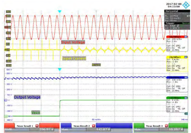
Figure 38 – 300 VAC, Full Load. Upper: V_{IN} , 200 V / div. Second: I_{IN} , 5 A / div. Third: V_{OUT} , 100 V / div. Lower: V_{AUX} , 5 V / div, 50 ms / div.
