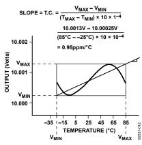
Figure 12. Typical AD588BQ Temperature Drift
