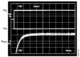
Figure 11. Turn-On with  $CN = 1 \mu F$
