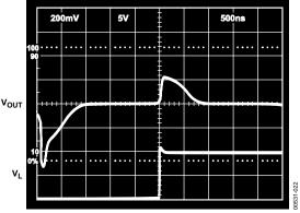
Figure 22. Large-Scale Transient Response
