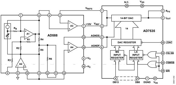
Figure 32. AD588/AD7535 Connections
