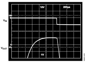
Figure 31. Output Amplifier Step Response Using Figure 30 Compensation
