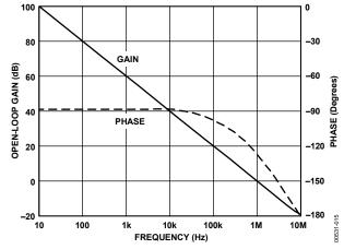
Figure 15. Open-Loop Frequency Response (A3, A4)
