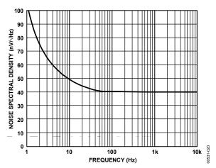
Figure 20. Input Noise Voltage Spectral Density
