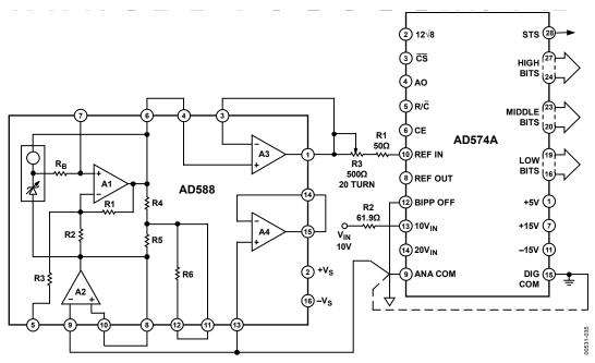
Figure 35. AD588/AD574A Connections
