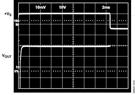
Figure 10. Extended Time Scale Turn-On
