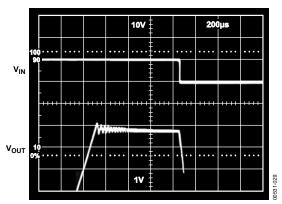
Figure 29. Output Amplifier Step Response,  $C_L = 1 \mu F$
