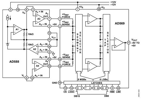
Figure 33. High Accuracy ±5 V Tracking Reference for AD569 Rev. G | Page 15 of 20
