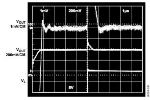
Figure 24. Transient Response 5 mA to 10 mA Load
