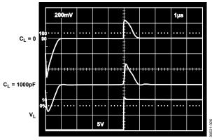
Figure 26. Output Response with Capacitive Load
