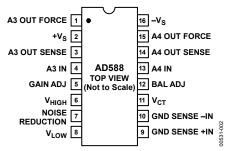
Figure 2. Pin Configuration
