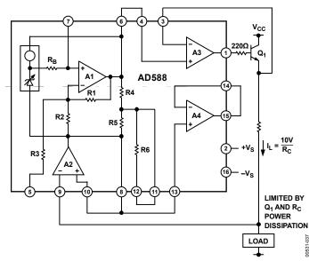
Figure 37. Boosted Precision Current Source
