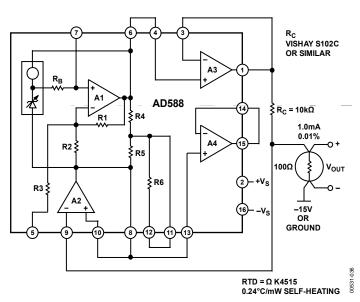
Figure 36. Precision Current Source for RTD
