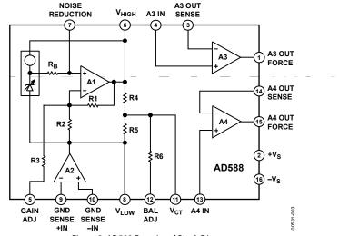
Figure 3. AD588 Functional Block Diagram
