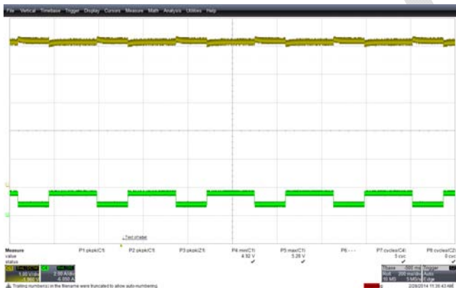
Figure 23 – Transient Response, 230 VAC, 800 mA to 1600 mA. Upper: V_{OUT} 1 V / div. Lower: I_{OUT} 2 A, 200 ms / div.
