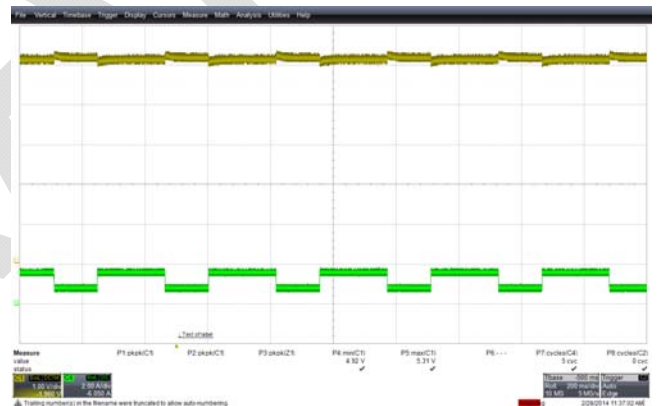
Figure 24 – Transient Response, 265 VAC, 800 mA to 1600 mA. Upper: V_{OUT} 1 V / div. Lower: I_{OUT} 2 A, 200 ms / div.
