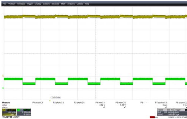
Figure 21 – Transient Response, 90 VAC, 800 mA to 1600 mA. Upper: V_{OUT} 1 V / div. Lower: I_{OUT} 2 A, 200 ms / div.
