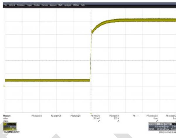
Figure 18 – Start-Up Profile, 115 VAC. Full Load. 1 V, 50 ms. / div.
