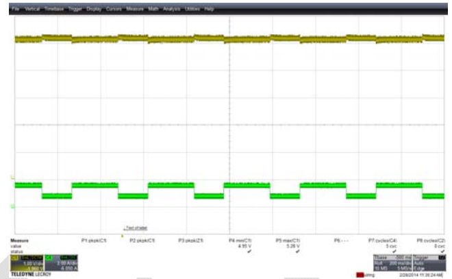
Figure 22 – Transient Response, 115 VAC, 800 mA to 1600 mA. Upper: V_{OUT} 1 V / div. Lower: I_{OUT} 2 A, 200 ms / div.
