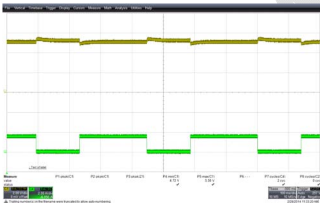
Figure 27 – Transient Response, 230 VAC, 20 mA to 1600 mA. Upper: V_{OUT} 1 V / div. Lower: I_{OUT} 2 A, 100 ms / div.
