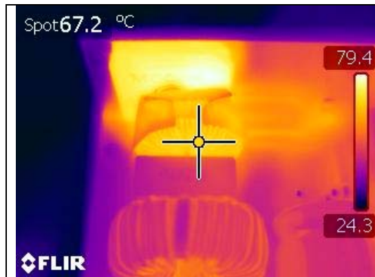
Figure 55 - Differential Mode Choke (L4), 115 VAC Input, 100% Load, Room Temperature.
