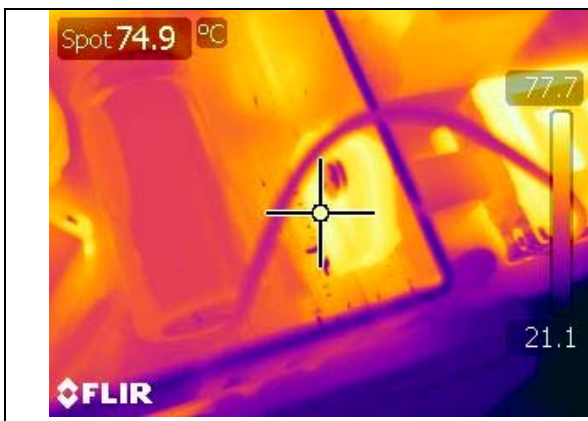
Figure 49 – LLC IC (U3), 90 VAC Input, 100% Load, Room Temperature.
