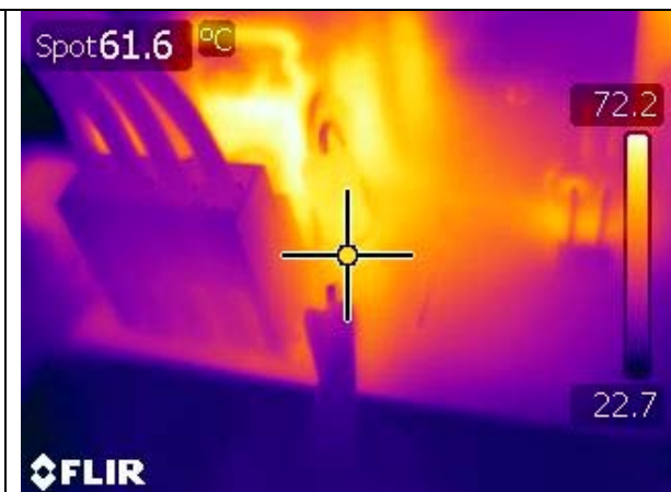
Figure 62 – Current Sense Resistor (R916), 115 VAC Input, 100% Load, Room Temperature.
