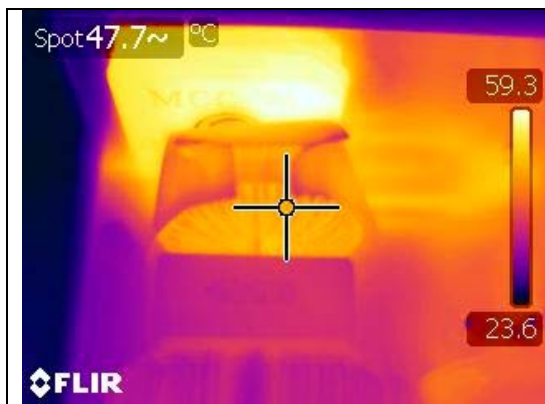
Figure 65 - Differential Mode Choke (L4), 230 VAC Input, 100% Load, Room Temperature.
