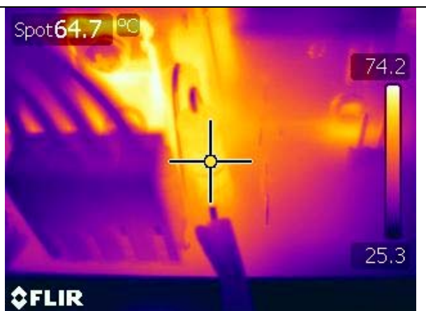
Figure 72 – Current Sense Resistor (R916), 230 VAC Input, 100% Load, Room Temperature.
