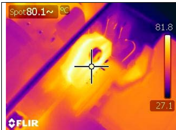
Figure 47 – PFC IC (U7), 90 VAC Input, 100% Load, Room Temperature.
