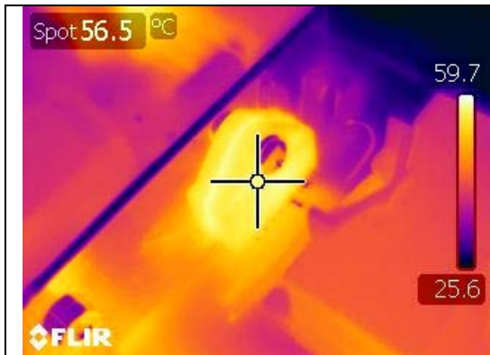
Figure 67 – PFC IC (U7), 230 VAC Input, 100% Load, Room Temperature.
