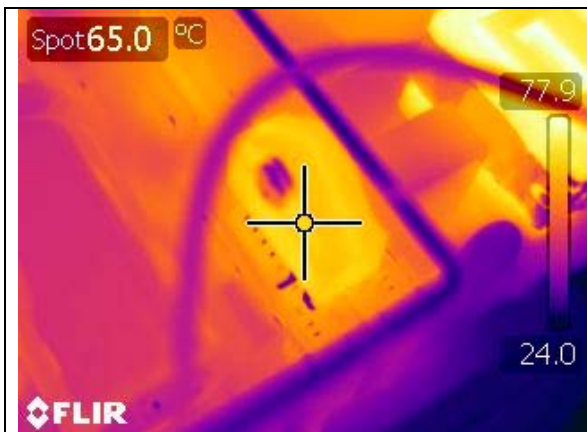
Figure 59 – LLC IC (U3), 115 VAC Input, 100% Load, Room Temperature.
