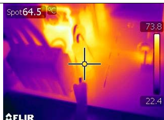
Figure 52 – Current Sense Resistor (R916), 90 VAC Input, 100% Load, Room Temperature.
