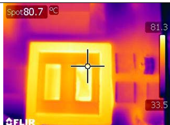
Figure 50 – LLC Transformer (T2), 90 VAC Input, 100% Load, Room Temperature.
