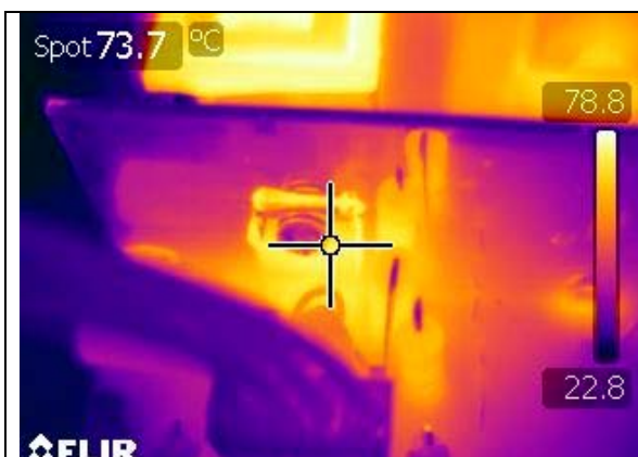
Figure 51 – Output Rectifier (D9), 90 VAC Input, 100% Load, Room Temperature.
