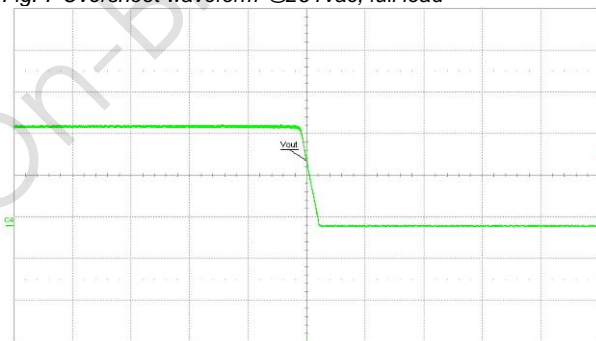
Fig. 7 Overshoot waveform @264Vac; full load
