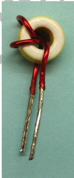
Figure 14 – Finished Part, Front View. Tin Leads to within ~ 1/8" of Toroid Body
