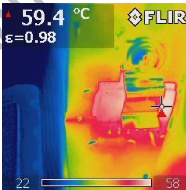
Figure 74 – Hiper LCS Case Temperature, 115 VAC, Full Load.
