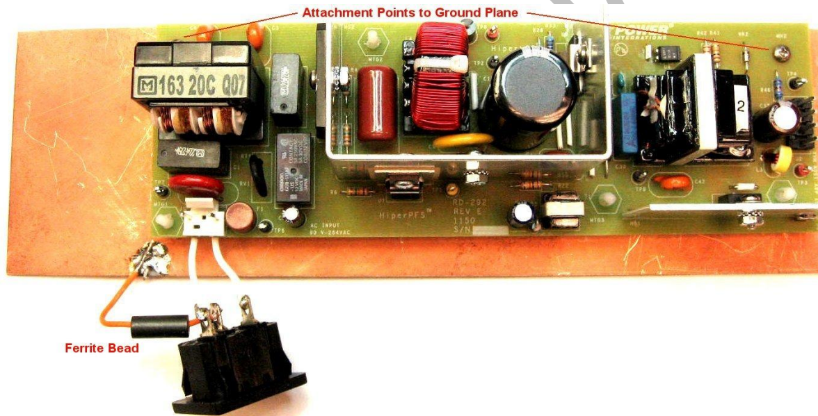
Figure 78 – RD-292 Set-up for EMI and Surge Testing.
