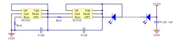
By cascade mode, two or more NU510 in series can absorb higher voltage variation in lighting system. Each NU510 can share about 8 volts redundant. The total voltage variation range that system can work is calculated by following equation.
