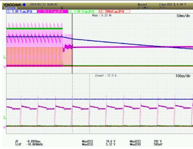
Figure 9. VIN = 90VAC, Short Protection
