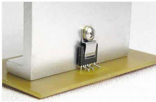
Figure 11: Metal eSIP strap mounting eSIP to a heatsink
