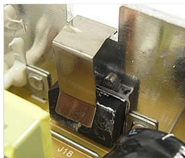
Figure 14: U-Clip securing an input bridge rectifier
