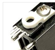
Figure 8: eSIP mounted to heatsink with Mini Strap (showing package details)
