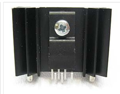
Figure 5: Plastic eSIP Strap Mounting eSIP to a Standard TO-220 Heatsink
