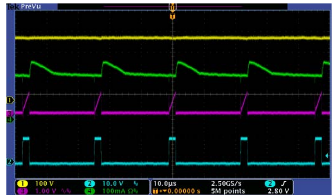
CH1: VBULK CH2: GATE CH3: CS CH4: IOUT
