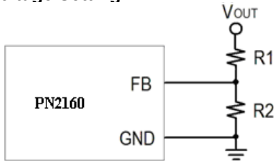
Figure 1: Output Voltage Setting
