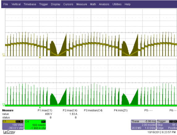
Figure 40 – 135 VAC, 60 Hz Output Short Condition. Upper: V_{DRAIN} , 100 V / div. Lower: I_{DRAIN} , 500 mA, 2 ms / div.
