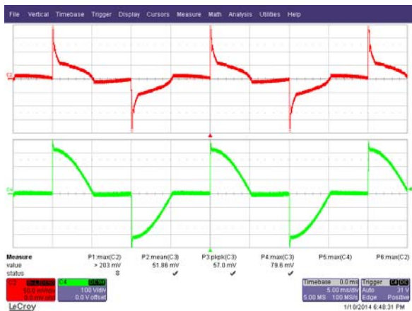
Figure 48 – 90° Conduction Angle. Upper: I_{IN} , 50mA / div. Lower: V_{IN} , 100 V, 5 ms / div.
