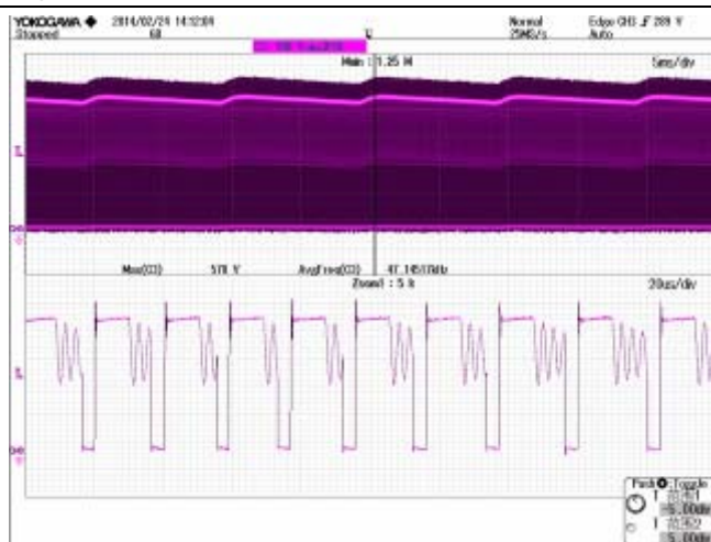
Figure 11. VIN = 264 VAC, Vds max=578V
