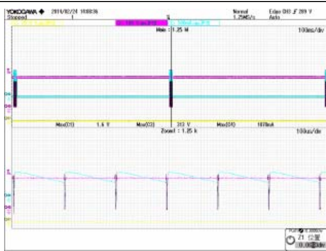
Figure 9. VIN = 176 VAC, LED Short, Vds_max=313V
