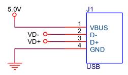
The EST5198B can detect the D+ line and D- line voltages automatically and provide the correct signals on the D+ and D- pins for the different USB portable device to fast charge.
