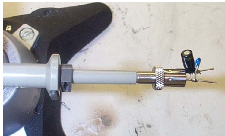
Oscilloscope Probe with Probe Master 5125BA BNC Adapter. (Modified with wires for probe ground for ripple measurement, and two parallel decoupling capacitors added)
