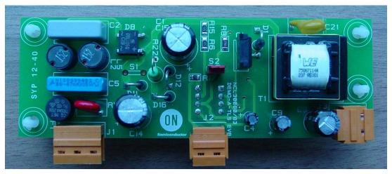
Figure 3. Photograph of the Top Side of the Valley Fill EVB
