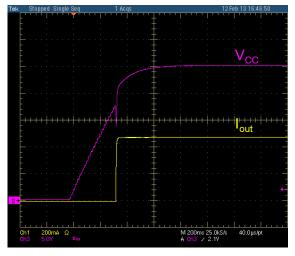
Figure 13. Startup Waveforms 230 V rms
