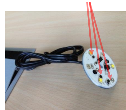
iML LED Driver ICs on Light Engine
