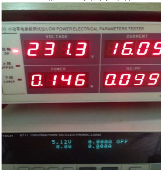
AC230V输入空载待机损耗
