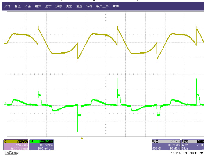
CH1: Input Voltage, CH4 : Input Current
