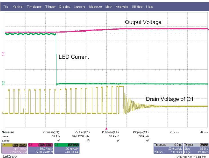
Fig. 6: Open LED Protection (20µs/div)
