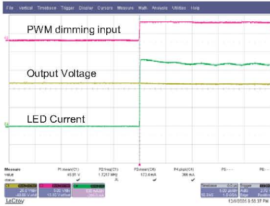
Fig. 9a: Rise time of LED Current at 40V output (5 \mu s/div)
