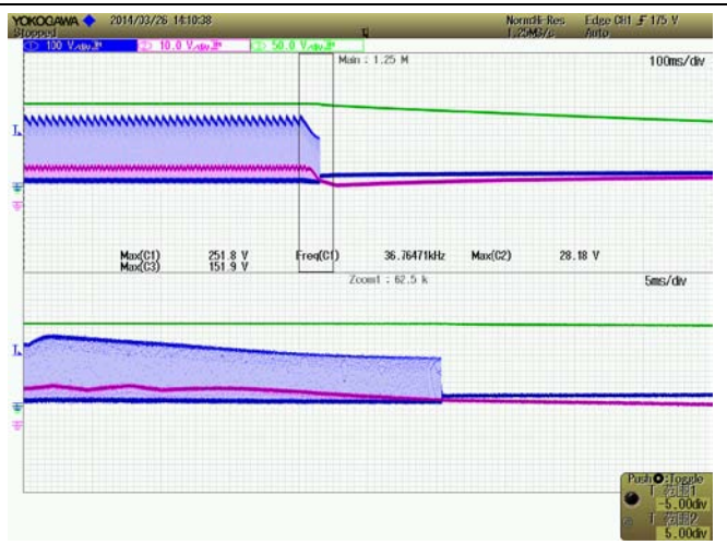
Figure 3. VIN = 176VAC, power off
