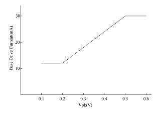
Figure 6: Base Drive Current vs VPK
