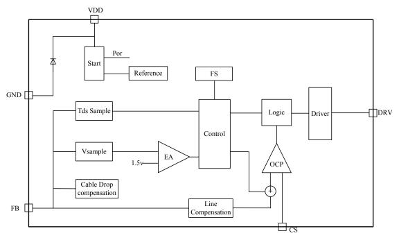
Figure 2: BF1565 Functional Block Diagram
