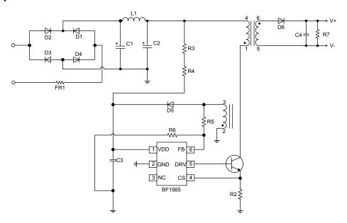
Figure 1: BF1565 Typical Application Circuit
