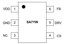
Figure 3: BF1565 Pin Configuration
