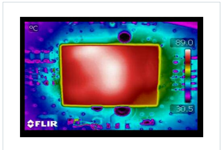
Figure 20 — Thermal Image (V_{IN} = 48\text{ V}, I_{OUT} = 5\text{ A}, CR, 0\text{ LFM Evaluation PCB})
