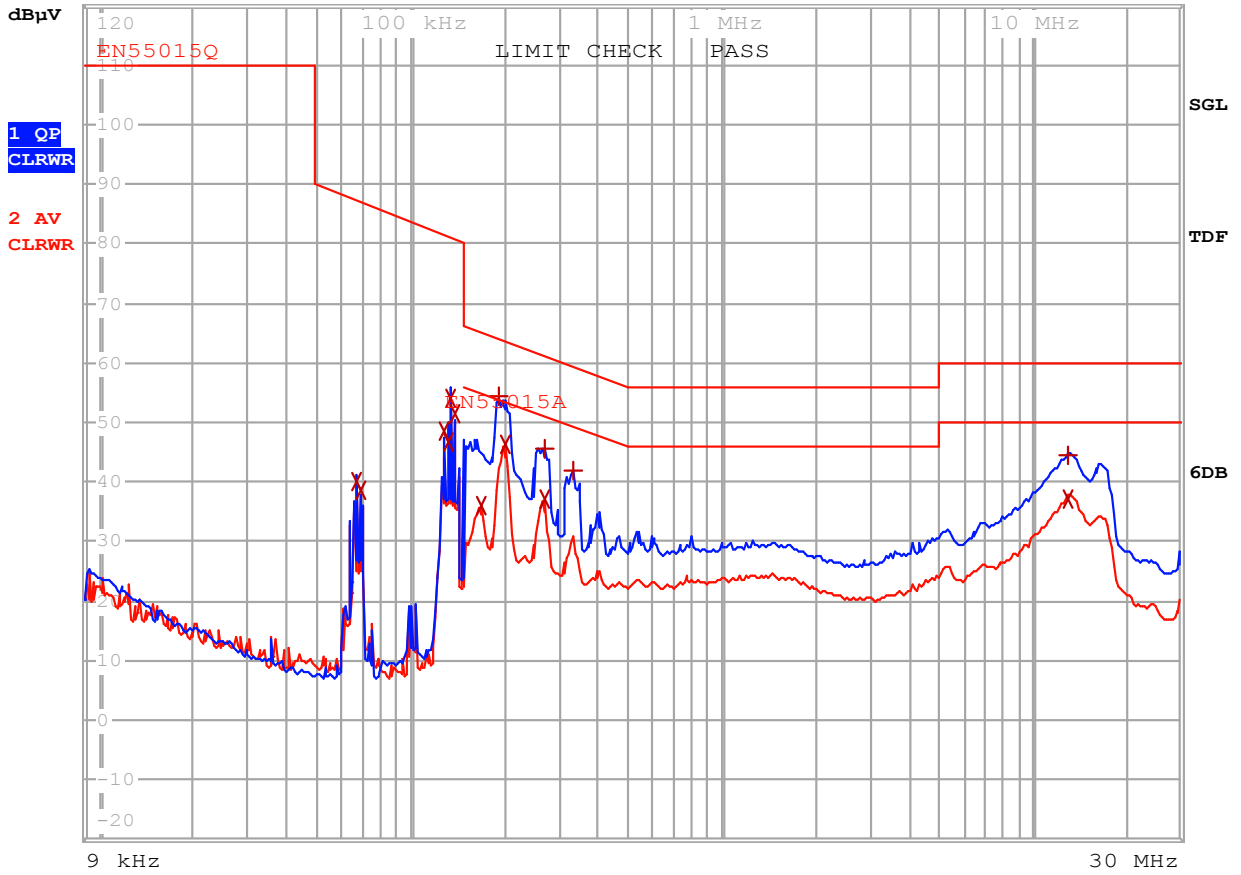
Figure 39 – Conducted EMI, Maximum Steady-State Load, 230 VAC, 60 Hz, and EN55015 Limits. 2-Wire Configuration (L-N).
