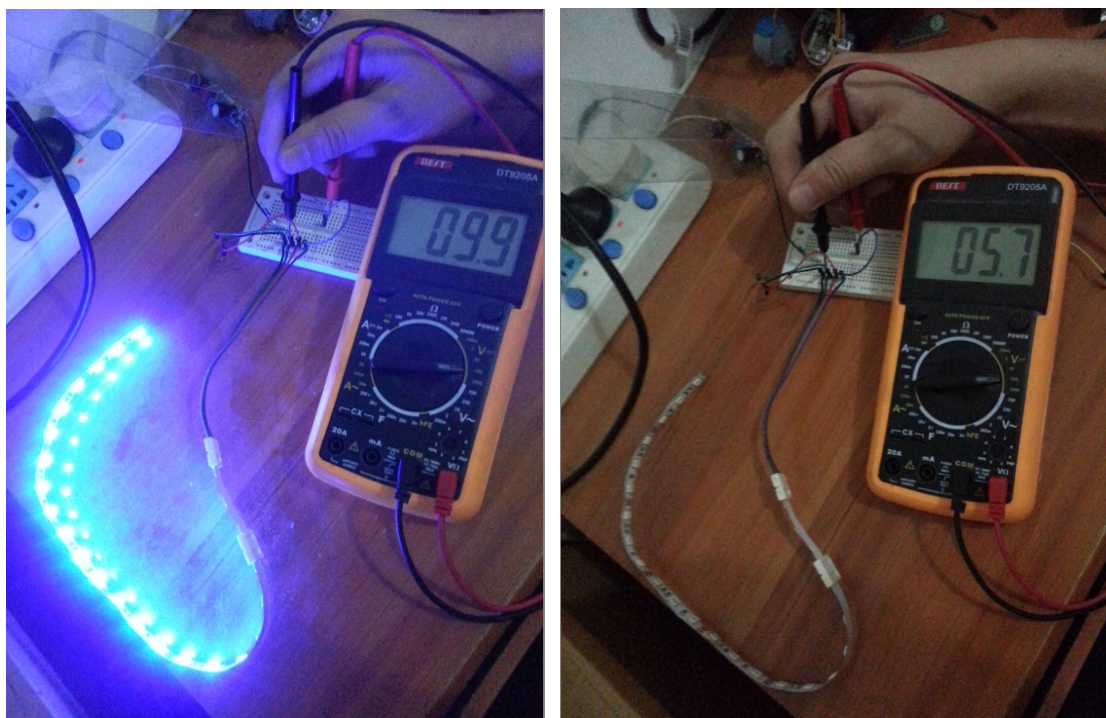
左：接入 LED 灯带，输出电压 9.9V
