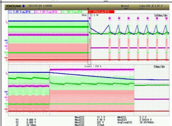
Vin=230Vac 输出短路，Vds_max=522V
