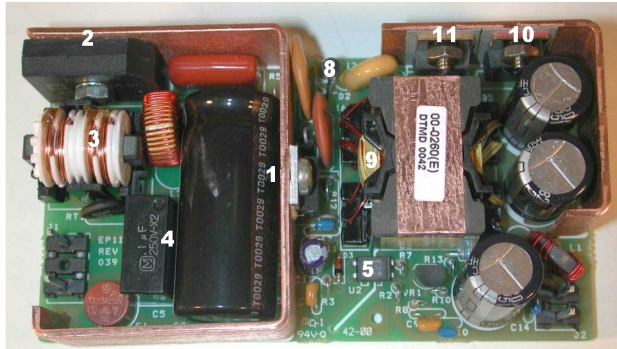
Figure 11 - Location of board mounted thermocouples
