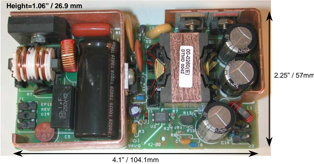
Figure 2 - EP11 Populated Circuit Board (dimensions include heat spreader not shown)
