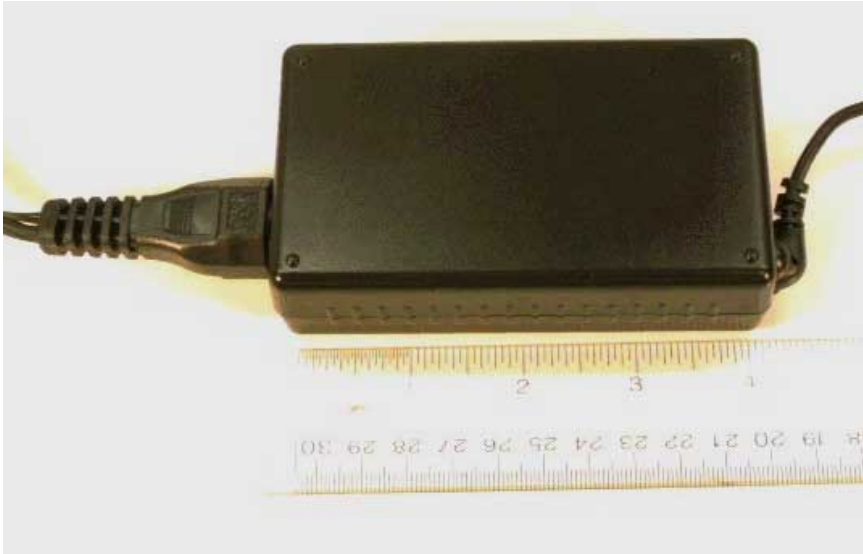
Figure 1 - EP11 Inside Commercial Laptop Enclosure (4.25 x 2.5 x 1.2" / 108 x 64 x 30mm – external diemnsions)
