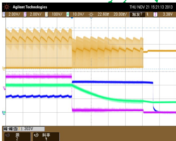
Fig.15 Short waveform@90Vac/60Hz,full load short
