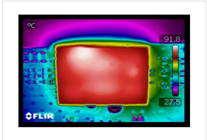
Figure 20 — Thermal Image ( V_{IN} = 28 V, I_{OUT} = 10 A, CR, 0 LFM Evaluation PCB)
