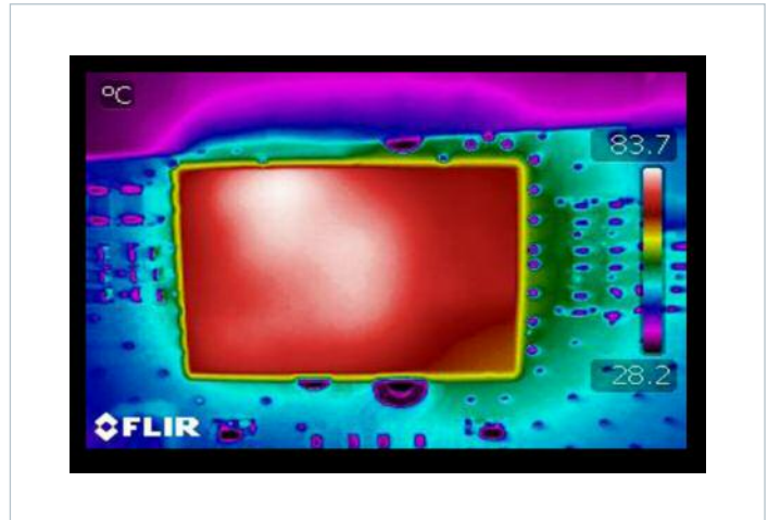
Figure 30 — Thermal Image ( V_{IN} = 28 V, I_{OUT} = 4.2 A, CR, 0 LFM Evaluation PCB)
