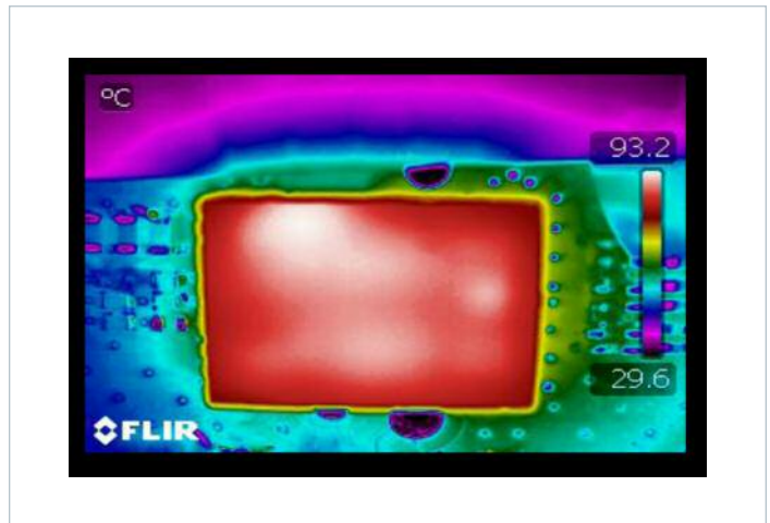
Figure 10 — Thermal Image ( V_{IN} = 24 V, I_{OUT} = 10 A, CR, 0 LFM Evaluation PCB)
